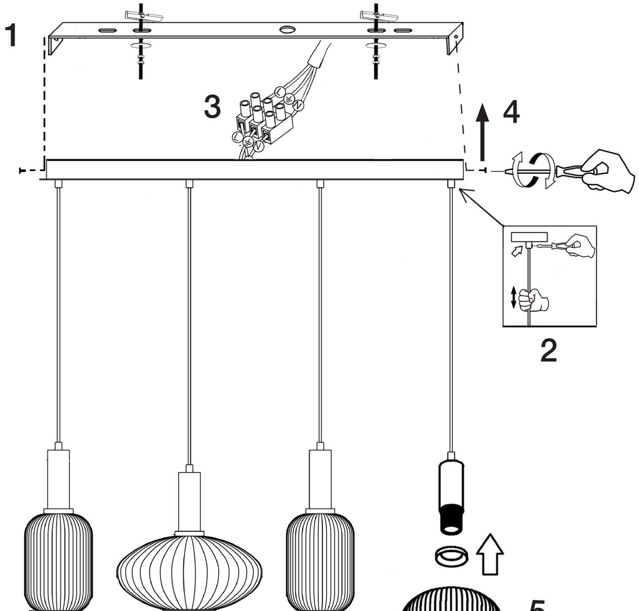
Adjust the length of the cables before installing. Place the glass shades once the lamp is installed in its final place.
